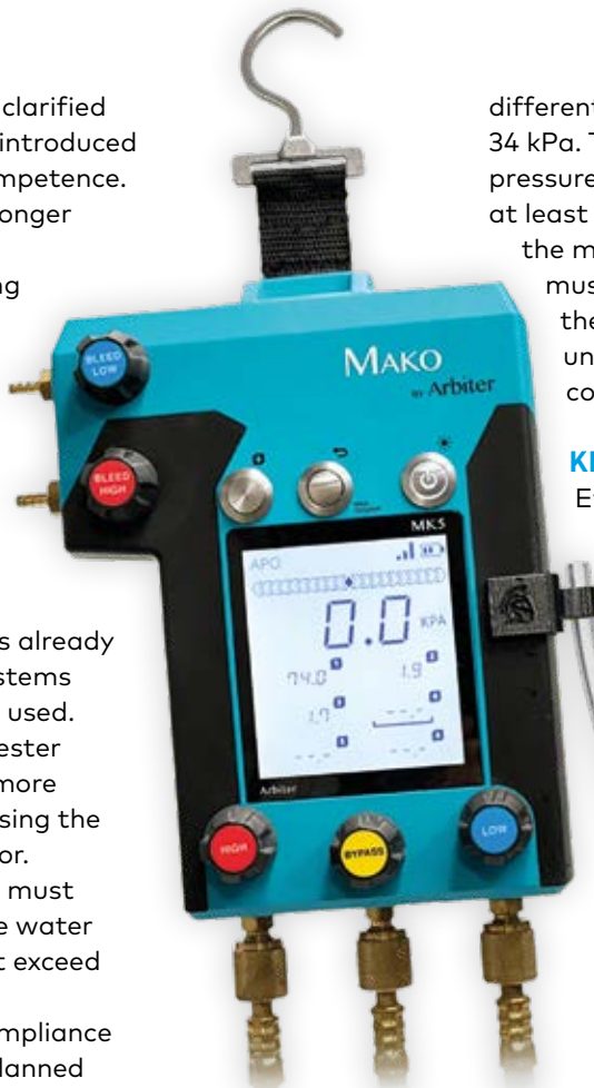
ABOVE: An RPZ valve test kit used to check RPZ valves are operating correctly
