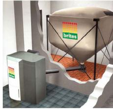
A wood pellet storage unit needs to be of sufficient strength to hold the pellets being stored (usually 4 tonnes). It needs to be waterproof (including damp), air tight and designed to reduce condensation.
