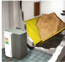
The fittings should be at chest height to be within the delivery driver's reach. An exit port should be fitted to allow the release of the delivery air. This needs a filter to reduce dust exiting the store.
